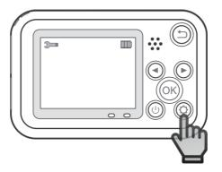
Press the setting key (wheel icon) to enter the setting interface / Click this button in the setting interface to withdraw action
