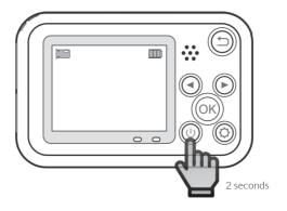
Press POWER BUTTON for 2 seconds to Turn off camera.
